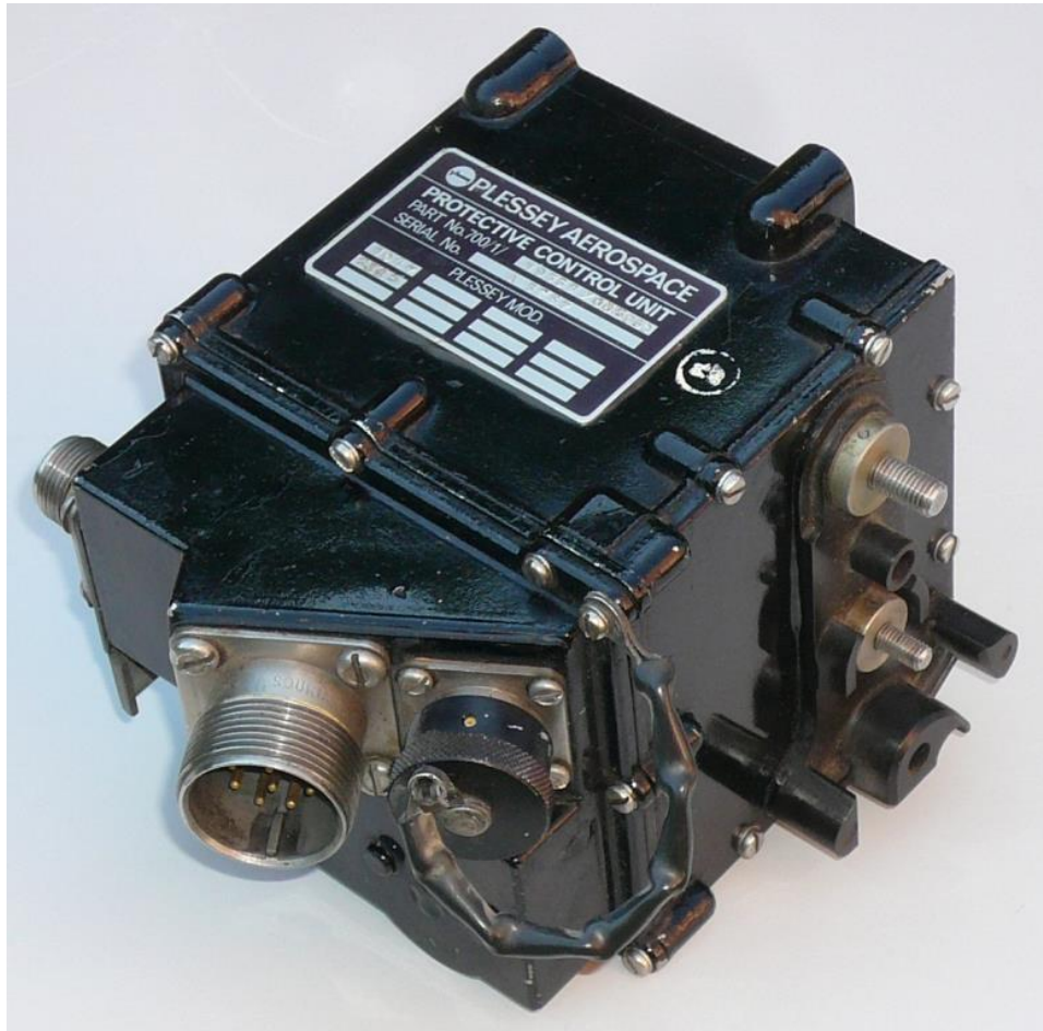
Electronic protection unit (RR Gem MK510)
