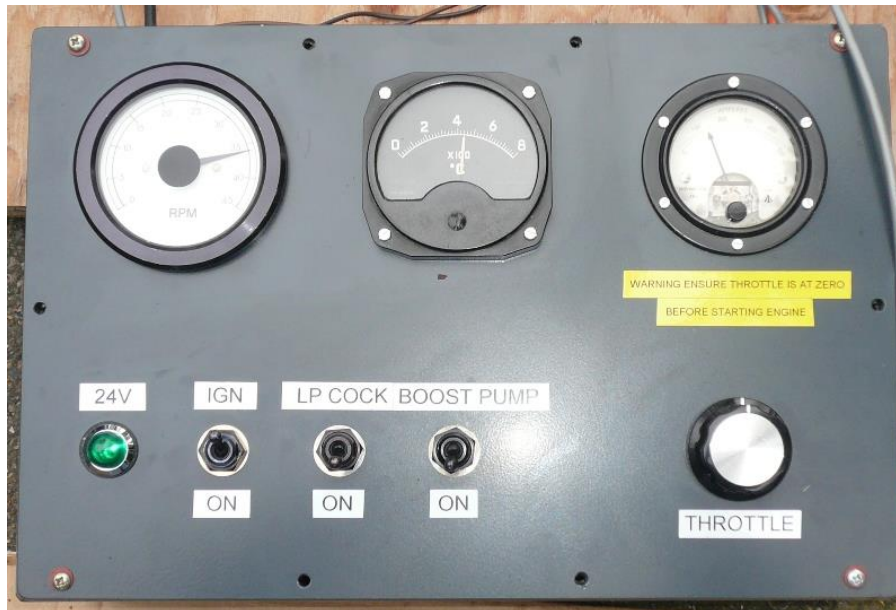
Simple test-set built to bench run a turbo-jet engine
