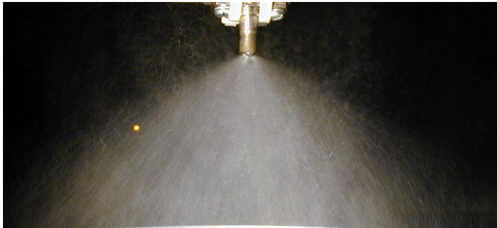
Spray pattern emitted by a single atomizing burner (Lucas)
