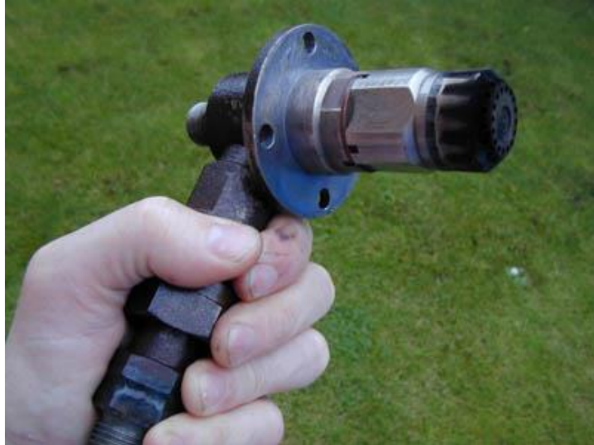
Burner unit intended for operation with natural gas (can type combustor)
