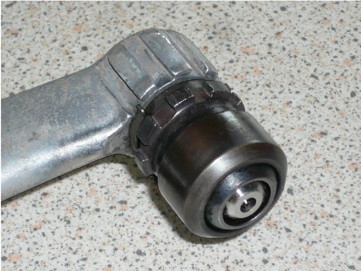
Duplex fuel burner nozzle (RR Spey)
