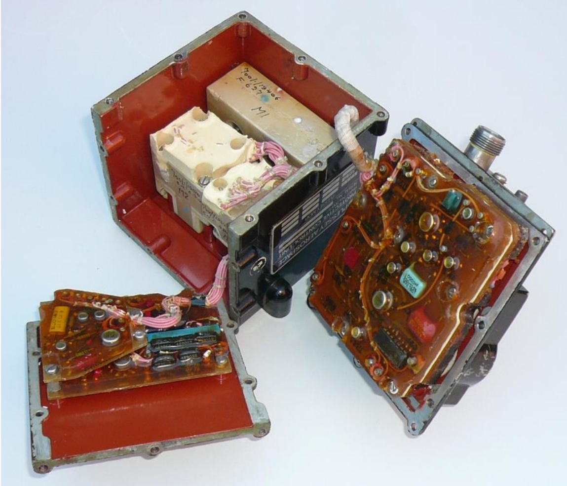
Inside engine protection unit showing circuit boards
