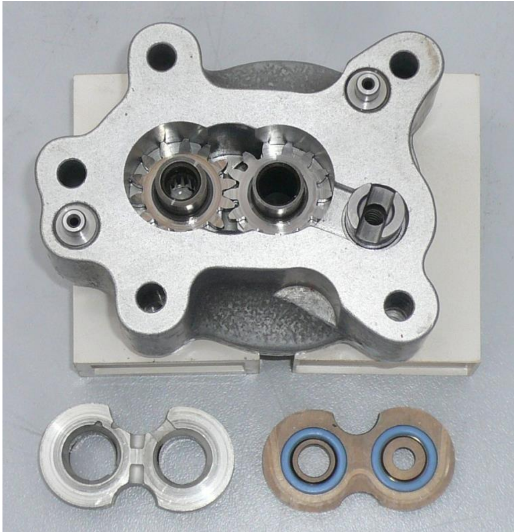
Disassembled gear type pump taken from small gas turbine engine
