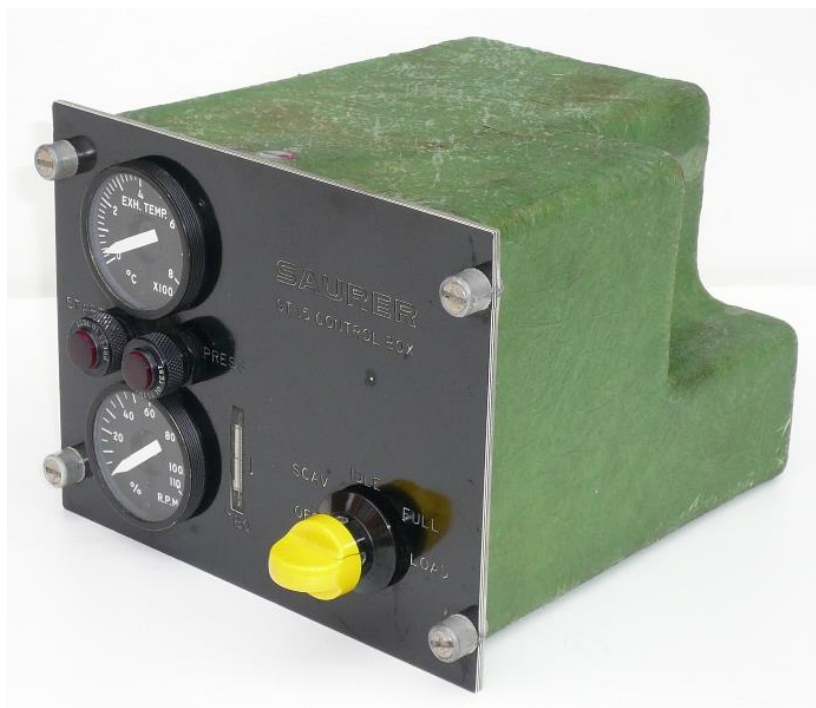
GT15 electronic control box and indicator panel
