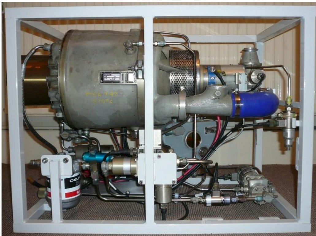
Microturbo fuel system featuring an electronic engine control unit
