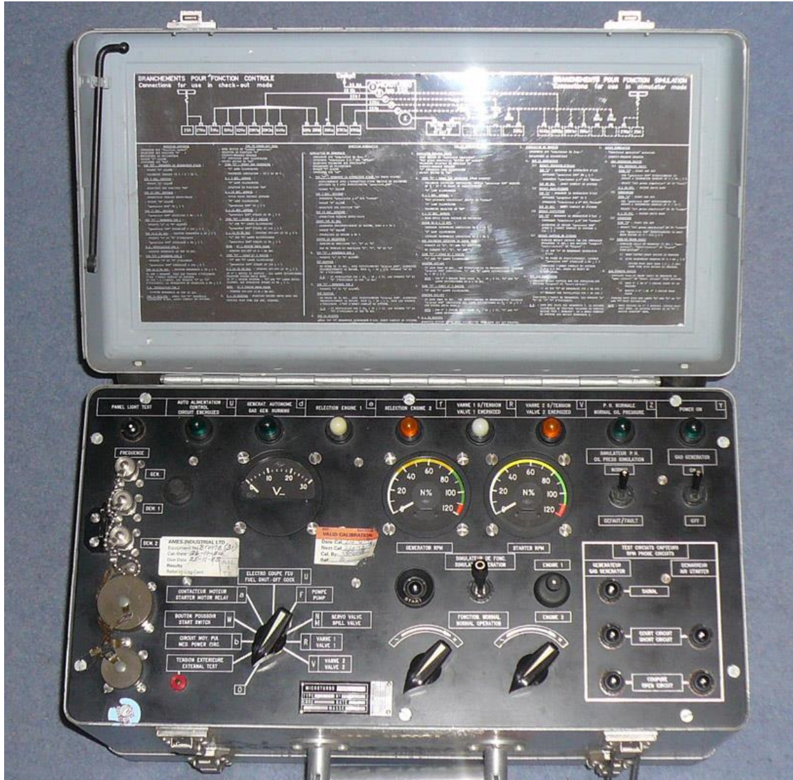
Test-set for gas turbine testing electronic control circuits.
