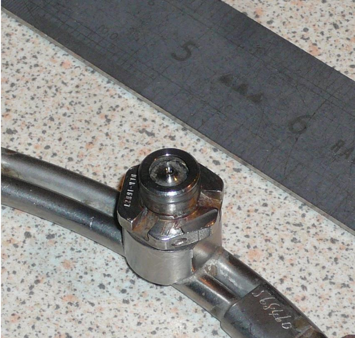
Simplex burner nozzle unit mounted in tubular distribution manifold (RR Gnome)
