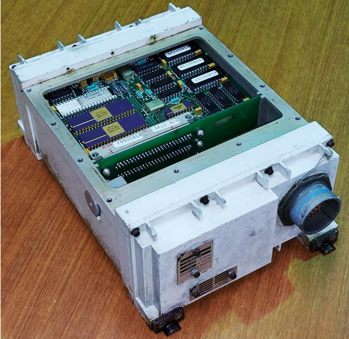
Lucas digital engine control unit (DCU)
