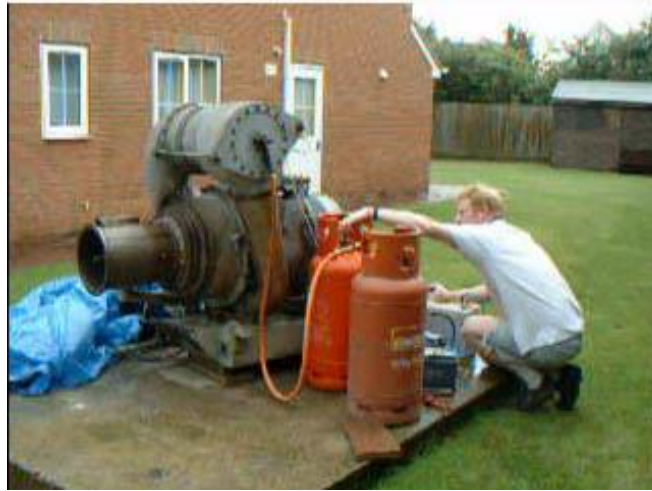
Test running a 250HP gas turbine fired by propane gas
