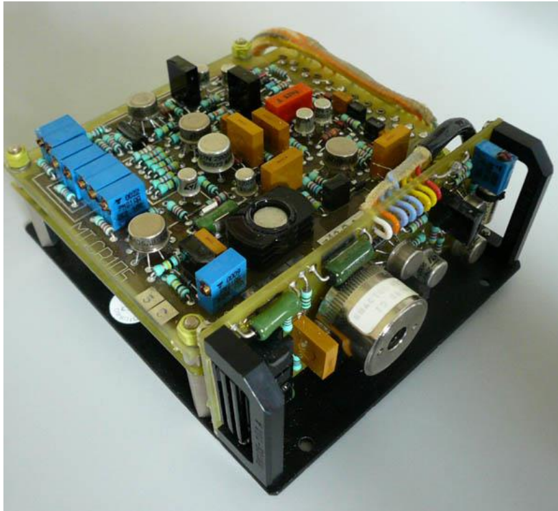
A typical gas turbine APU electronic control unit (ECU)
