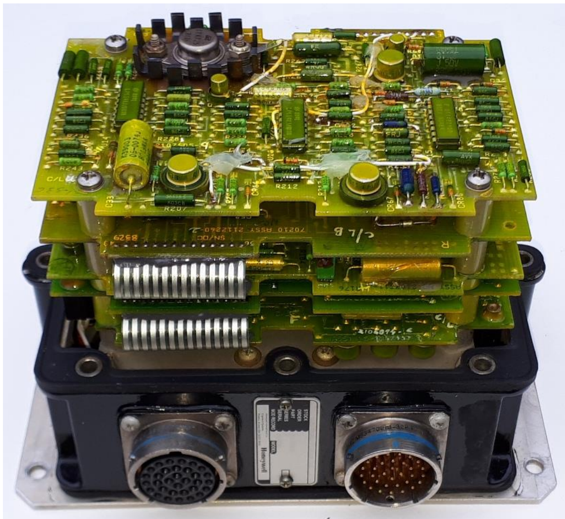
A Honeywell model 36 analogue engine control unit (ECU)
