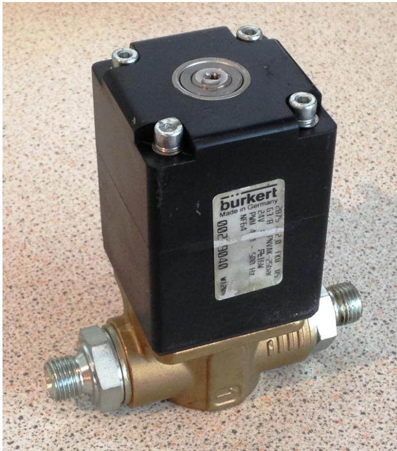
Solenoid operated proportional valve (Burkert)
