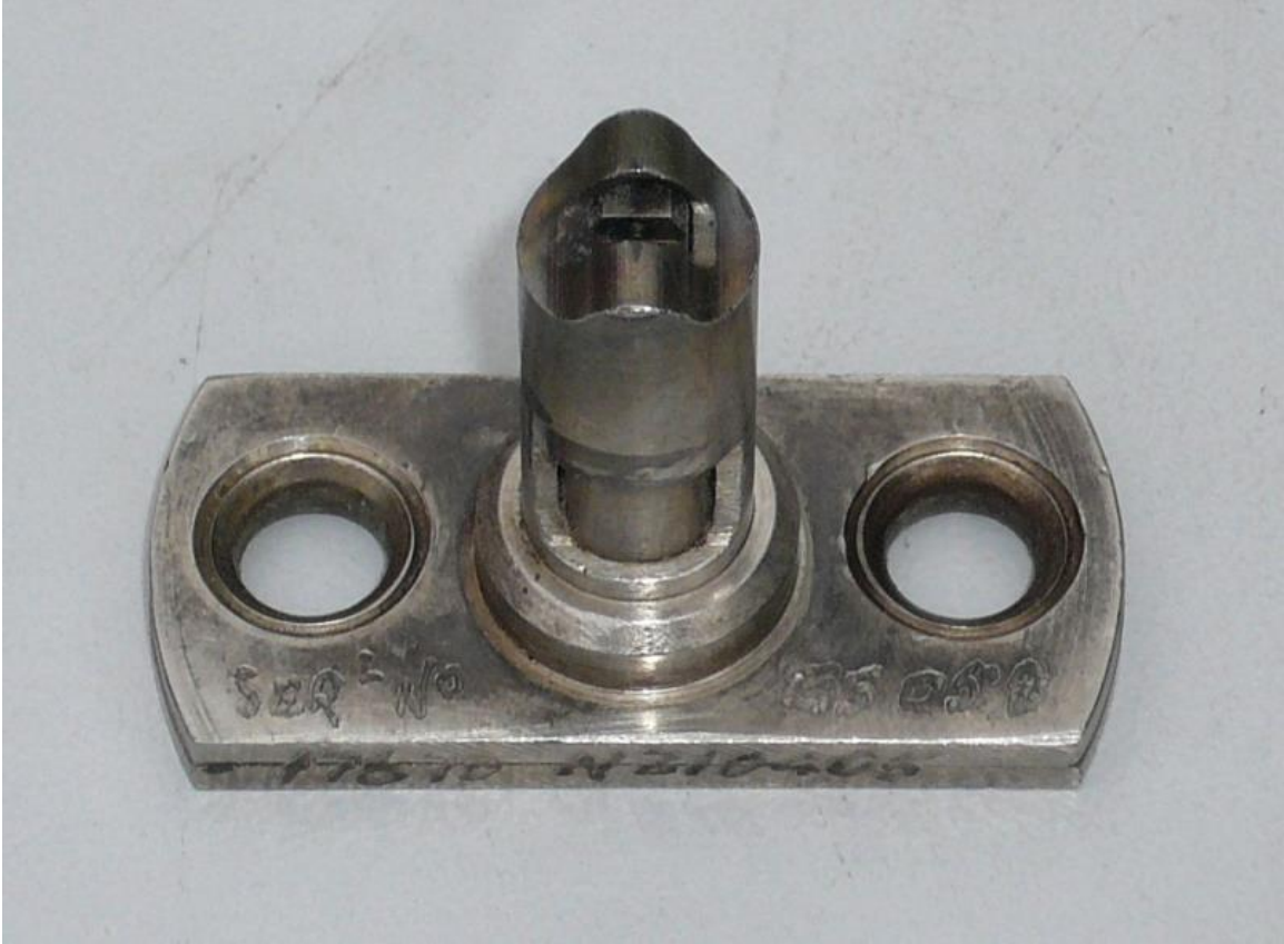
Miniature flat-fan atomizer taken from a small gas turbine engine (Rotax CT2023)
