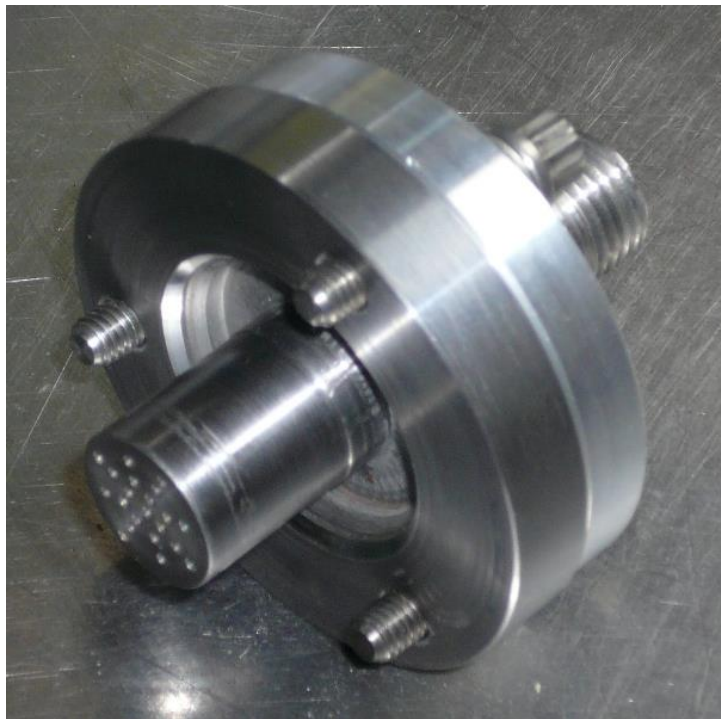
Manufactured experimental gas burner head unit (replaces liquid atomizer)
