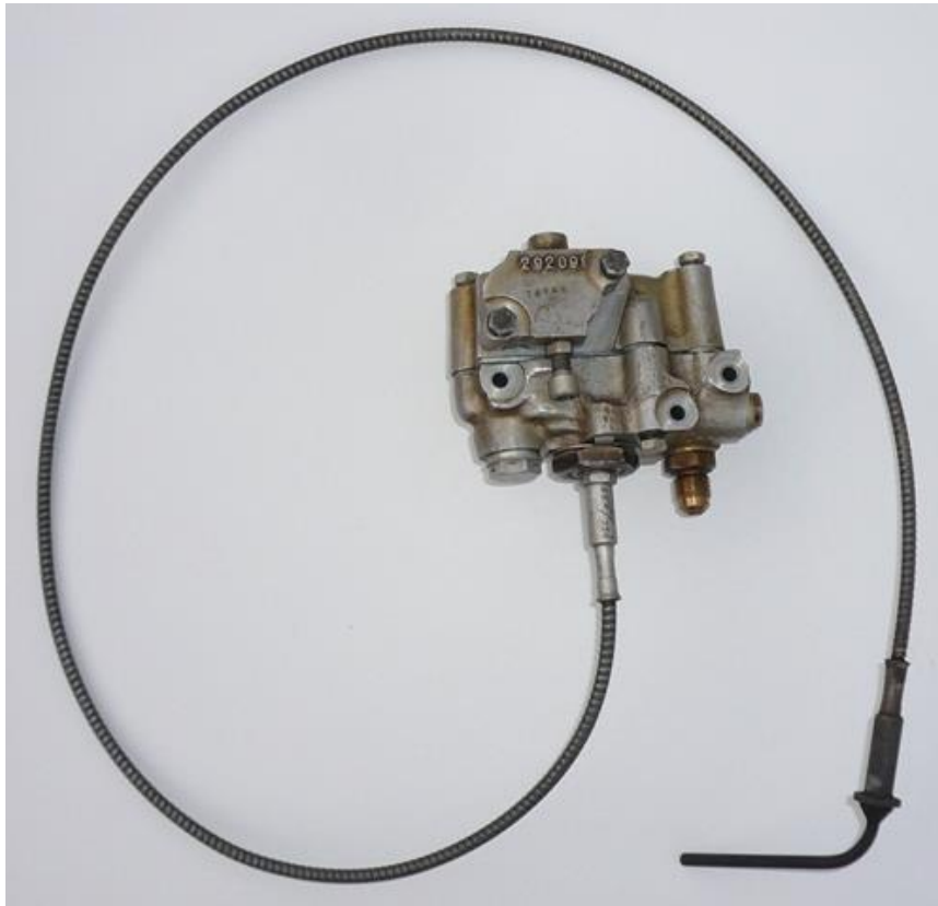
Temp limiter probe and fuel spill valve (Rover)
