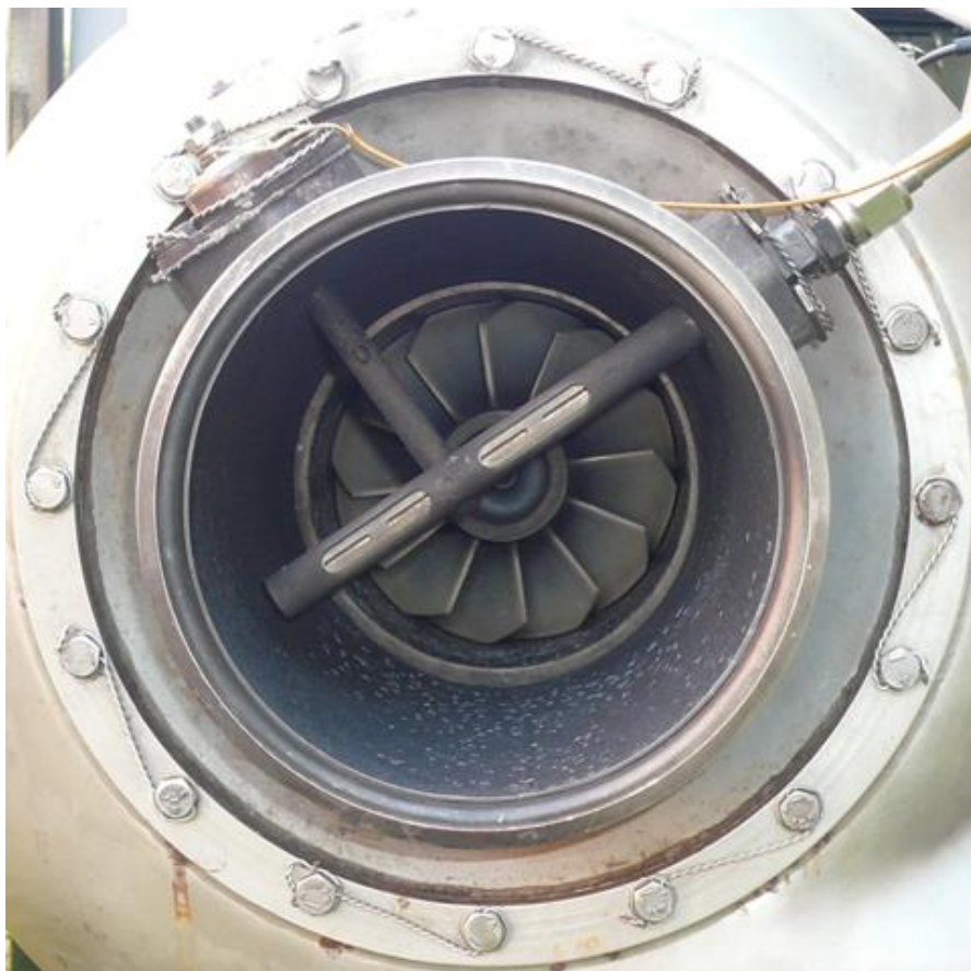
Picture Garrett temp limiter sensing valve
